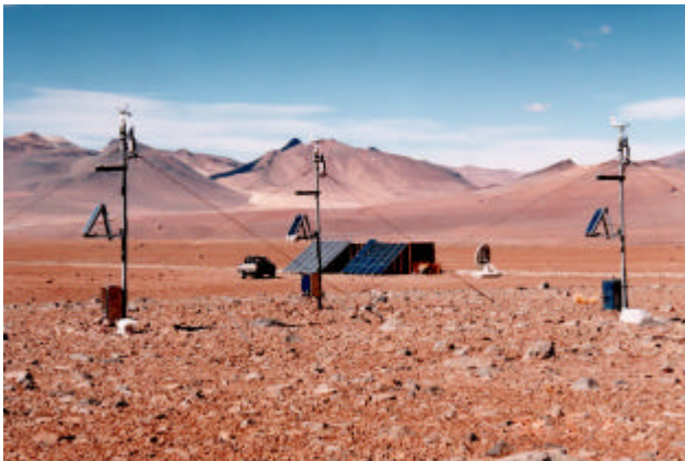
Fig. 4 Site testing instruments and containers at the 4800 m site of Pampa la Bola, Region II, Chile. Two containers equipped with solar panels and one of the element antennas of the radio seeing monitor can be seen in the background. Three weather stations under cross calibration are seen in the foreground.
